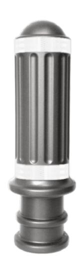
Bollard made of high and low-density compact polyethylene. Inner core made of recycled rubber which offers a high resistance to impacts. Two reflecting bands on top and bottom.
