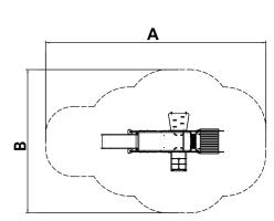
**Structure, Metal:** hot-dip galvanised and powder coated 80x80x2mm posts resistant to abrasion, corrosion and bad weather conditions. 2mm thick AISI 304 polished stainless steel slide surface curved and molded in one piece. Ø32mm protective bars made of AISI 304 stainless steel.
