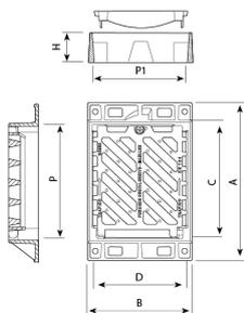
Tráfico D4 is designed to support heavy traffic. It is perfect for installing on roads with an ADT of 1.000-20.000, particularly road carriageways (including pedestrian streets), stabilised hard shoulders and parking areas for all manner of vehicles.
