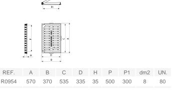
Imbornal is designed to support soft traffic. Perfect for installing on roads with an ADT of < 500, particularly hard shoulders and ditches.
