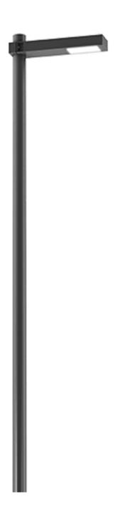
Pole made of laminated steel tube with a 200mm x 100 mm rectangular profile. Height from 4m to 7m. Can include one or two brackets (same or different height).
