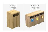
Litter bin made of pine wood treated in vacuum pressure autoclave Class IV against woodworm, termites and insects. Natural colour finish. Litter bin with lid so that water cannot enter the bag and door to facilitate the replacement of the bag. Opening on both sides. Stainless steel screws. Recommended anchoring: by means of three M8 expansion bolts depending on the surface and the project.
