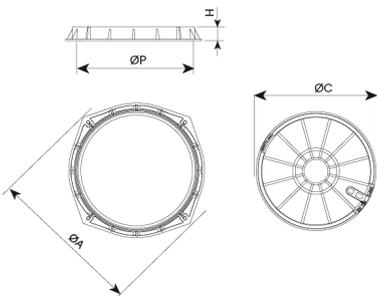
HRM D4 is designed to support soft traffic. It is perfect for installing on roads with an ADT of 500 a 1.000, particularly road carriageways (including pedestrian streets), stabilised hard shoulders and parking areas for all manner of vehicles.
