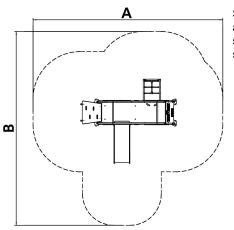
**Structure, Metal:** hot-dip galvanised and powder coated 80x80x2mm posts resistant to abrasion, corrosion and bad weather conditions. 2mm thick AISI 304 polished stainless steel slide surface curved and molded in one piece. Ø32mm protective bars made of AISI 304 stainless steel.
