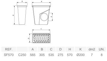
Delta is designed to withstand low traffic. Perfect for installing on roads with an ADT of 500 to 1,000, particularly hard shoulders and ditches.
