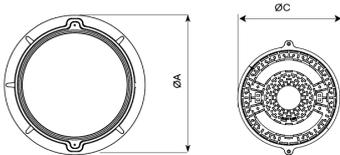
Compo C2 is designed to support soft traffic. Perfect for installing on roads with an ADT of 500 to 1.000, particularly hard shoulders and ditches.
