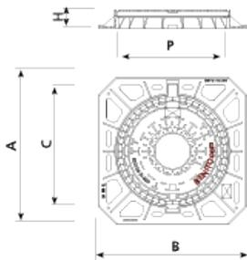
Hexa is designed to support medium traffic. It is perfect for installing on roads with an ADT of 1.000-20.000, particularly road carriageways (including pedestrian streets), stabilised hard shoulders and parking areas for all manner of vehicles.
