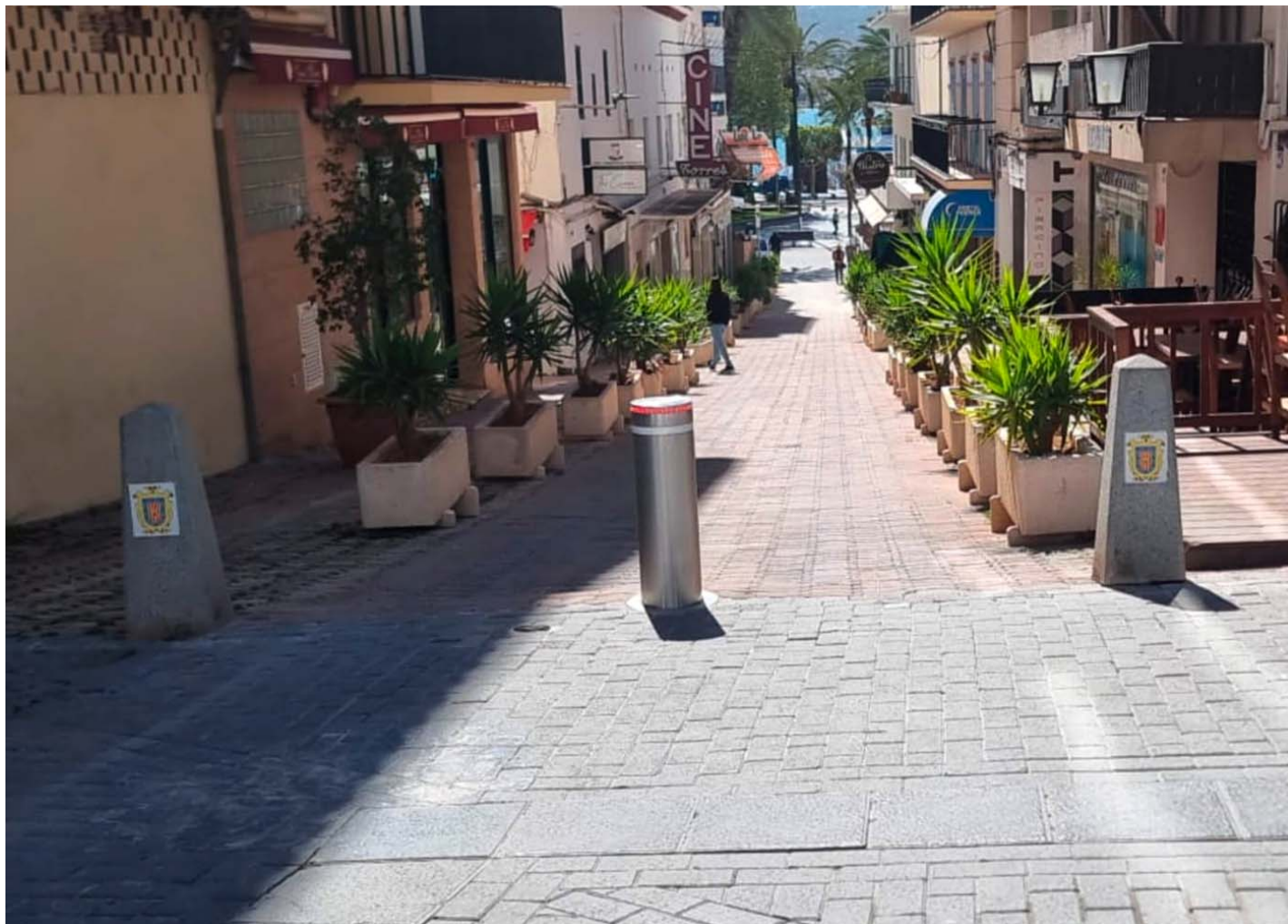
Automatic Telescopic Ø220 x 600 mm H6008
