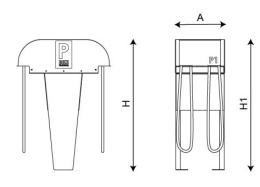
**BIT secure bike rack for two bicycles, managed via app.** It incorporates a double fixing chain with anti-scratch coating, protection box for the saddle, space for the helmet and electronic opening by means of a pivoting door. Recommended anchorage, by means of four M10 expansion bolts depending on the surface and project.
