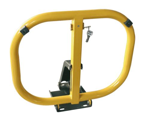
Bollard made of galvanised steel tube treated with Ferrus, a protective process that guarantees high resistance to corrosion. This treatment consists of three layers applied after shot cleaning all impurities: zinc plated, epoxy primer coating and yellow RAL 1021 polyester powder coating.
