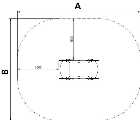
**Structure, Metal:** Ø35mm stainless steel AISI-304 posts. 2mm thick AISI 304 polished stainless steel slide surface curved and molded in one piece.
