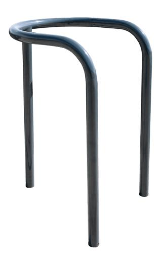
Protector for poles or trees made of steel treated with Ferrus, a protective process that guarantees high resistance to corrosion. Epoxy primer and grey RAL 7016 polyester powder coated finish.
